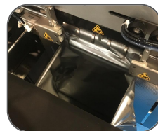
Easy load bag opener squares open and grips the bag
