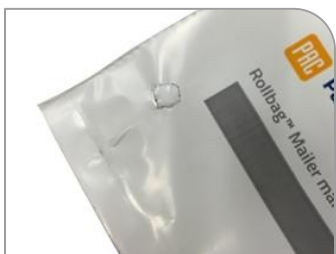
Adjustable Hole Punch —Pneumatic punch that puts a small perforated hole (flutter vent) in the bag, allowing for excess air to escape.
