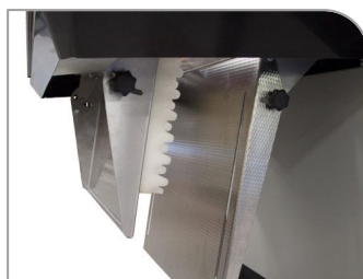
Air Expeller —The air expeller is a plate with a foam pad. This device presses against the bag prior to sealing, removing excess air.
