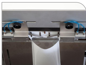
Seal Flattener Fingers —Seal Flatteners work to hold bag taut during sealing to minimize wrinkles. Also shown is the bag in open position before bag is stretched for sealing.
