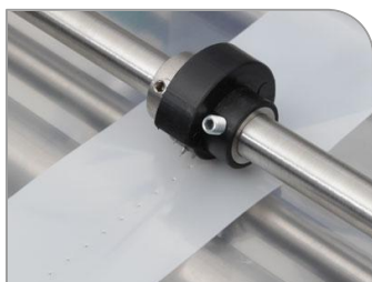
Film Perforator —The film perforator has an upper and lower assembly which creates a vertical perforation along the complete length of the bag. This perforation allows air to vent out of the bag after it has been sealed.
