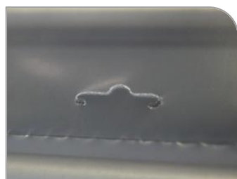
Seal Bar with Hang Hole —A seal bar that also creates a hang hole near the top of the bag to allow a package to be placed on a retail display hook.
