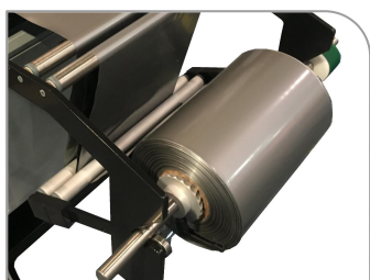
Bag Maker Assembly —The bag maker assembly allows the R3200 bagger to use poly tubing, in addition to pre-opened bags on a roll. With poly tubing the user can change the desired bag length at the push of a button, since the bag is made on demand. The assembly applies a bottom seal to the tubing, as well as perforates and opens the material, prior to loading. When using poly tubing the R3200 will run up to 40 bags/min (dependent on bag size, gauge, and product).
